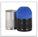
Manufacturer Description: The eXact iMpact™ 40mm Sponge Round is a point-of-aim, point-of-impact direct-fire round. This lightweight, high-speed projectile consisting of a plastic body and sponge nose that is spin-stabilized via the incorporated rifling collar and the 40mm launchers rifled barrel. The round utilizes smokeless powder as the propellant and, therefore, has velocities that are extremely consistent. Used for crowd control, patrol, and tactical applications.
